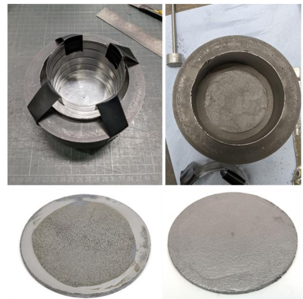
Figure 5. Clockwise from top left: SPS/FAST Ø80mm die filling with central Ø65mm tube, pure Ti-64 rim and central blended Ti-64 + \text{NaCl} sections after filling, the consolidated part encased in conductive graphite paper, the final part after the graphite paper is removed.
