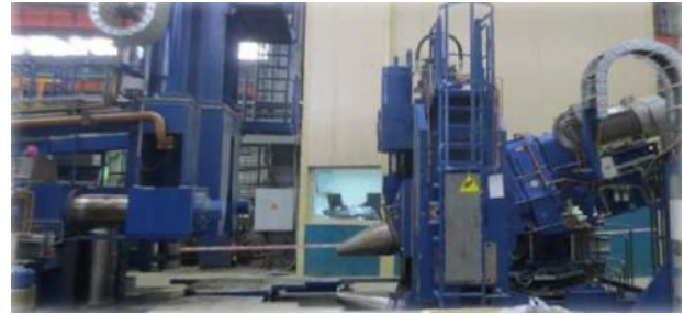
Figure 5. Ring rolling mill RAW 400/200-3500/800
