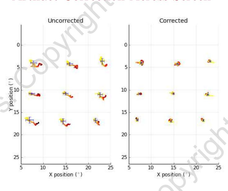
The pupil artifact is viewing location dependent. We corrected for arbitrary screen coordinates by measuring at 9 locations in a 3x3 grid pattern, and interpolating model fit parameters between these locations using quadratic bivariate spline interpolation.
